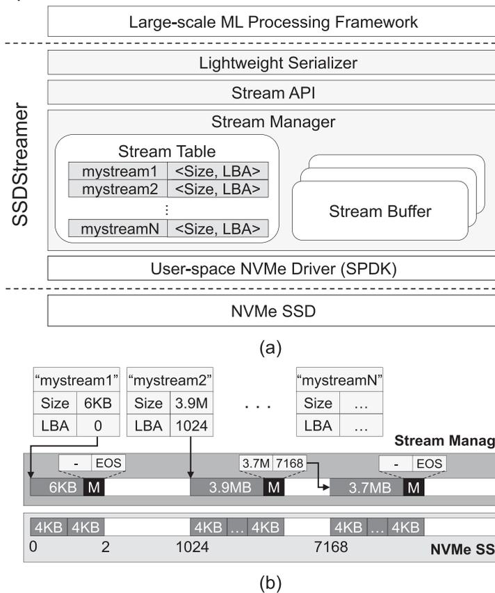
**Figure 3.** (a) SSDStreamer system stack. (b) Stream metadata structure and sblock chaining.
