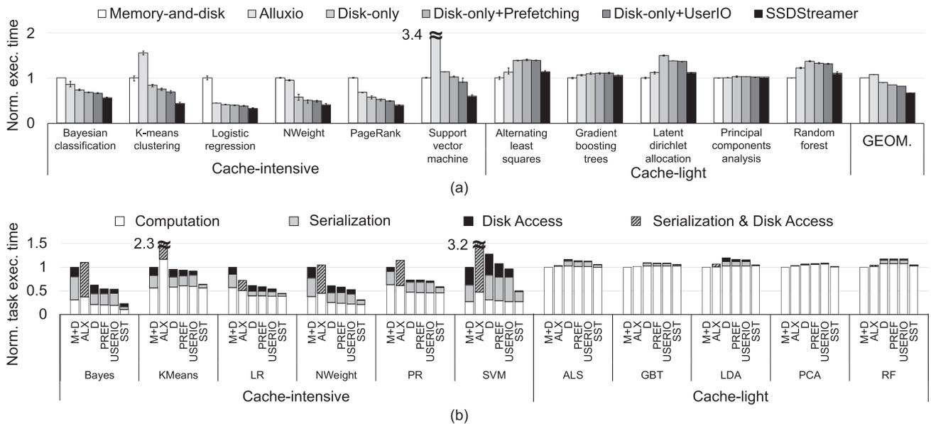
**Figure 5.** (a) Normalized execution time. (b) Normalized task execution time breakdown.
